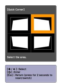
Using the  $[ \bigcirc ]$ ,  $[ \bigcirc ]$ ,  $[ \bigcirc ]$ , and  $[ \bigcirc ]$  buttons on the remote control, or the  $[ \square ]$ ,  $[ \square ]$ ,  $[ \triangleleft ]$ , and  $[ \triangleleft ]$  buttons on the control panel, correct the position of the corner.
