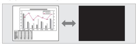
Each time you press the [A/V Mute] button or open/close the lens cover, A/V Mute turns on or off.
