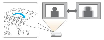
EB-W16 comes with a built-in function to help make accurate focus adjustments.
