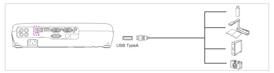
When the USB device is connected, you can project files on the USB memory or digital camera using PC Free.
