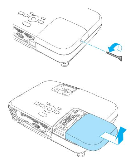
3 Loosen the two lamp fixing screws.
