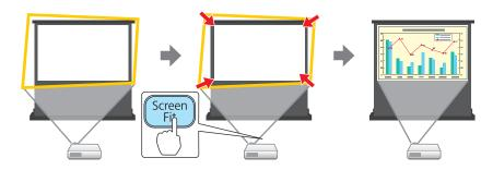
You can use Screen Fit to correct the projected image under the following conditions.
