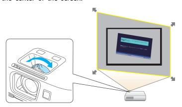
If the yellow frame is still within the screen frame even after adjusting the zoom ring to its maximum size, try moving the projector further away from the screen.
