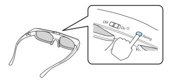
The indicator flashes alternately green and red. If pairing is successful, the indicator turns green for ten seconds and then turns off.
