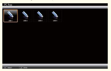
• To display the Select Drive screen, position the cursor on **Select Drive** at the top of the file list screen, and then press the [] button.
