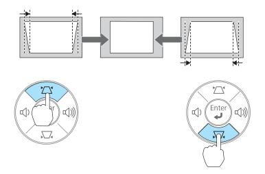
Press the [♠] or [♠] button to correct horizontal distortion.
