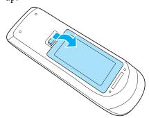
Replace the old batteries with new batteries.
